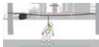
PN3000 a length ranging from 5m to 20m. Only used by one person at the same time EN 795:1996, Class B
