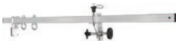
PN802 Installed on door frame of width from 60 to 125cm Only used by one person at the same time Provided with bag: BG34 EN 795: 2012 Type B
