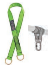
PN804 2m Polyester Webbing D-Ring on both ends. Min. Breaking Strength: 18kN EN795:2012 Type B
