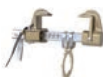
SA08 (Mini) Flange width from 75 to 150mm Min. Breaking Strength: 23kN EN795:2012 Type B
