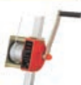
PN801絞動器 Galvanized Steel Wire Rope of Dia. 4.5mm Length of Cable 20m Capacity : 135kg Standard : EN 1496 CLASS A
