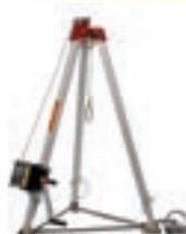
PN800三腳架(7 ft.) Adjustable height from 1.15m to 2.15m Maximum Load Capacity : 500kg Standard : EN795 TYPE B
